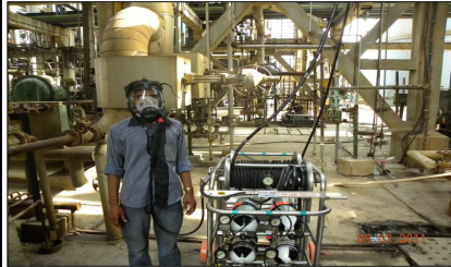
Six cylinders (each cylinder of 1200 litres and 30 minutes working duration) Breathing Apparatus with 40 m hose
